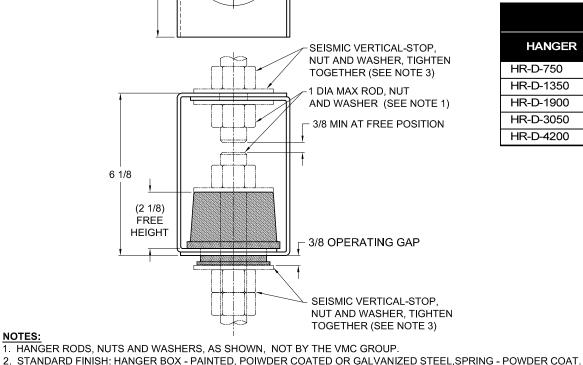
3. VERTICAL LIMIT-STOP HARDWARE REQUIRED FOR SEISMIC APPLICATIONS, NOT BY THE VMC GROUP.
